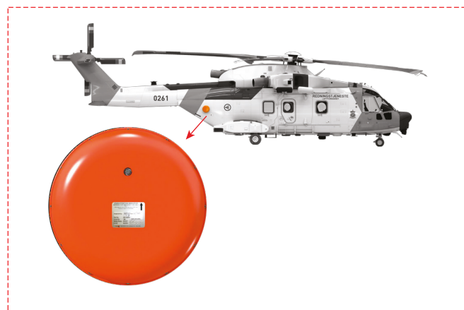
Crash Position Indicator, safety distance 1,2m
